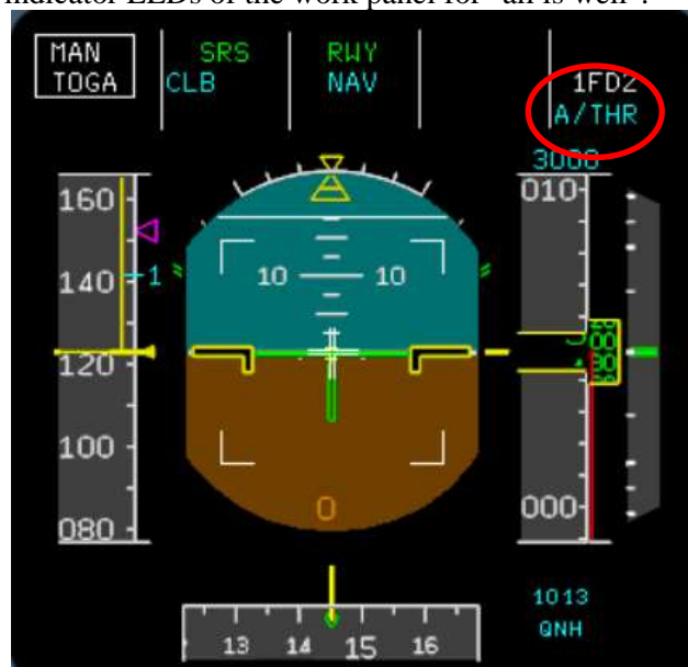
Figure 7: Auto-Thrust indicator on the A320 primary flight display
