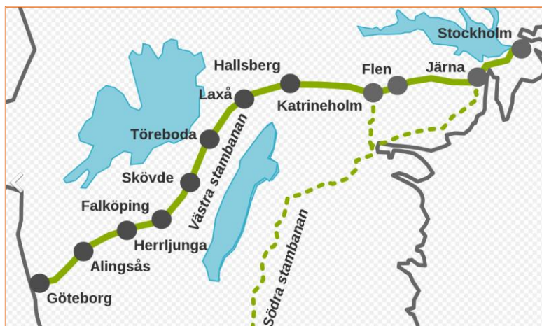
Figure 2. The Western Main Line in Sweden connects Stockholm and Gothenburg and is a 455 km long ballasted double track with 60E1 and 50E3 rail and Monoblock concrete sleepers.
