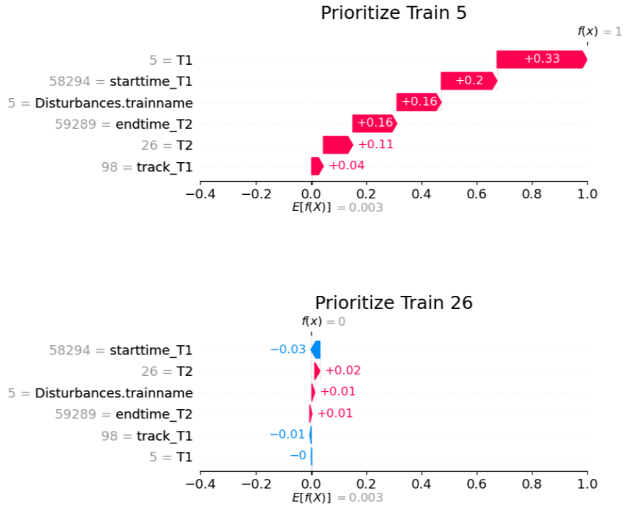
Figure 18: Scenario 345: A waterfall plot that explains why the model suggests prioritizing Train 5 to resolve potential conflict 1 at track 2 of section MLB-SÖLA
