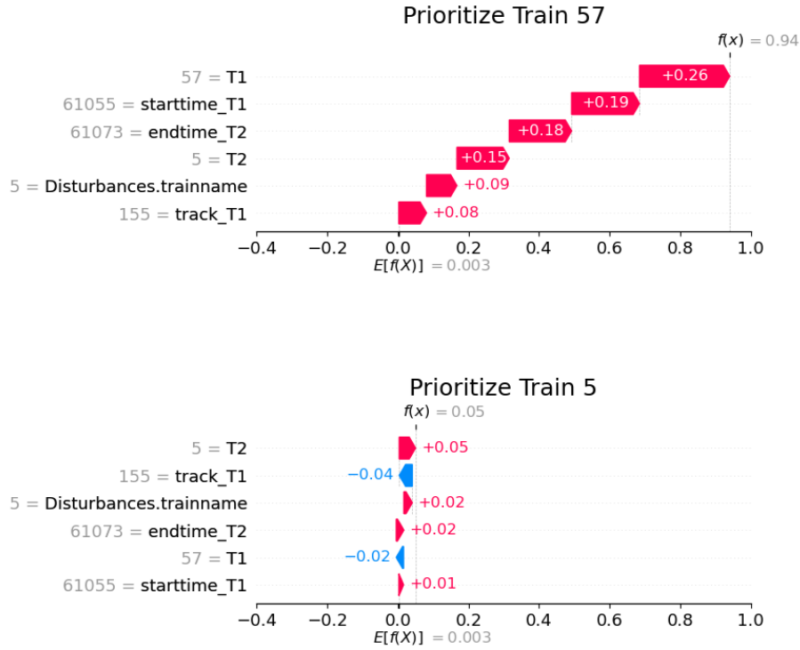
Figure 21: Scenario 345: A waterfall plot that explains why the model suggests prioritizing Train 57 to resolve potential conflict 4 at track 2 of section ÅKN-ÅK
