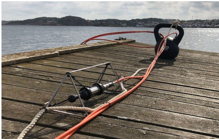
Figure 3. Mounted hydrophone and bottom weight.
