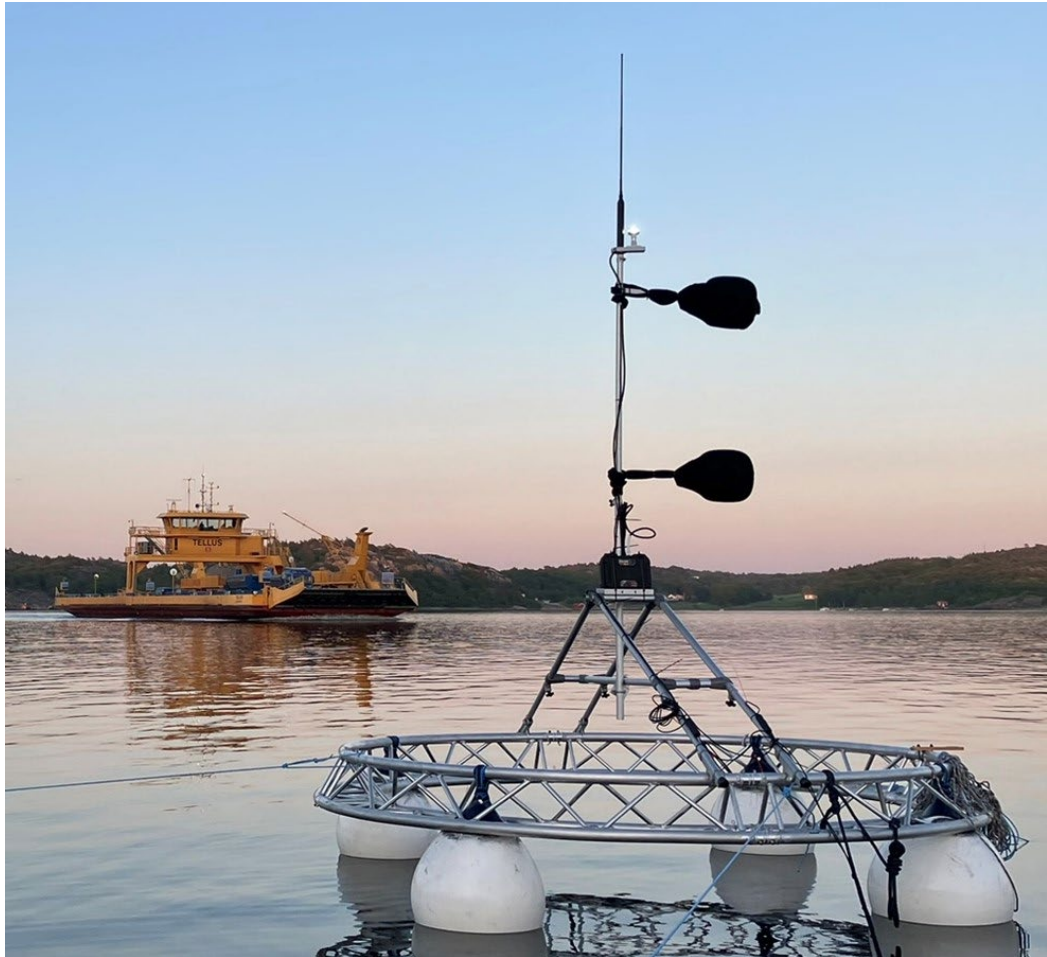
Figure 1. The 'SilentRaft' floating measurement platform with the ferry Tellus approaching.
