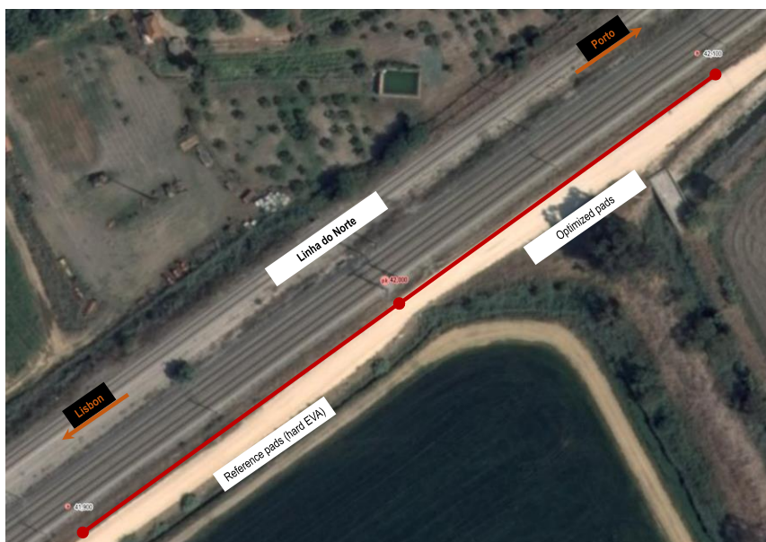
Figure 42: Overview of the measurement site at IP
