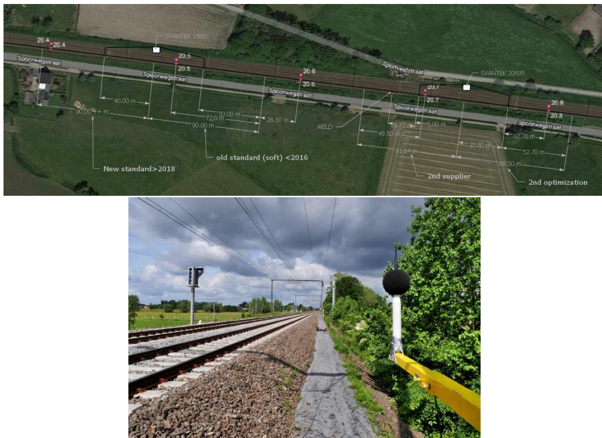
Figure 37: Top: overview of the test track at INFRABEL, Bottom: a microphone at the opposite side of the test track at INFRABEL
