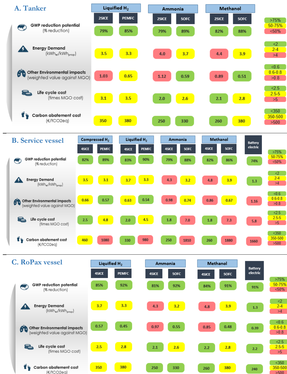
Figure 1010: LCA and LCC results from the study for case vessels simplified into three color scales based on relative values A) results for the Tanker, B) results for the Service vessel, and C) results for the RoPax vessel.
