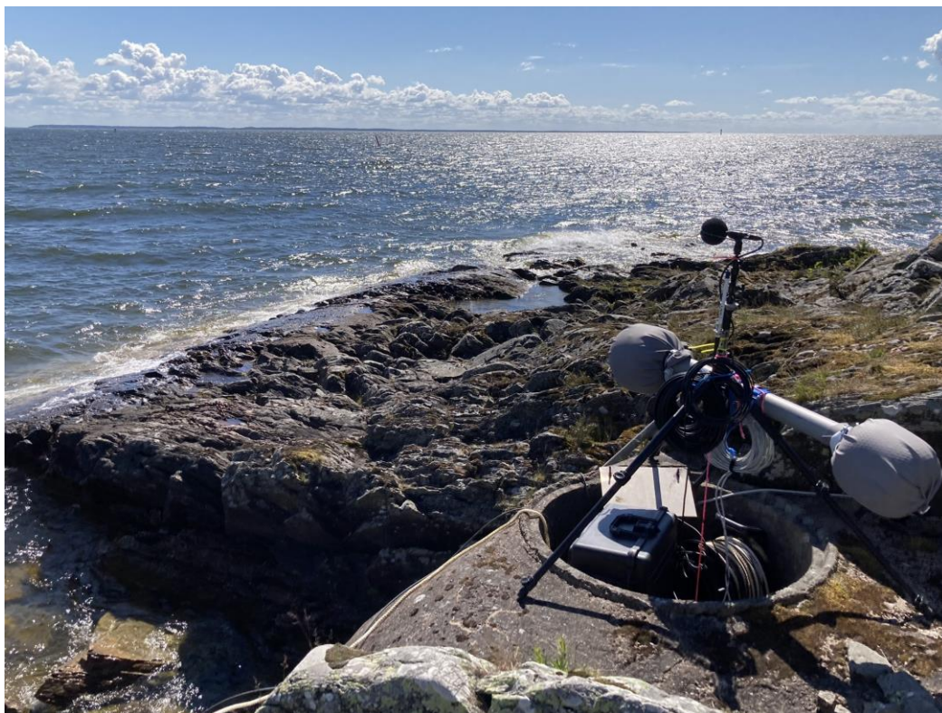
Figure 12. The wide-band microphone and the low-frequency sensor mounted on a tripod at Stångudden on Lurö. The cassion lighthouse Pålgrunden can be seen on the horizon above the tripod.
