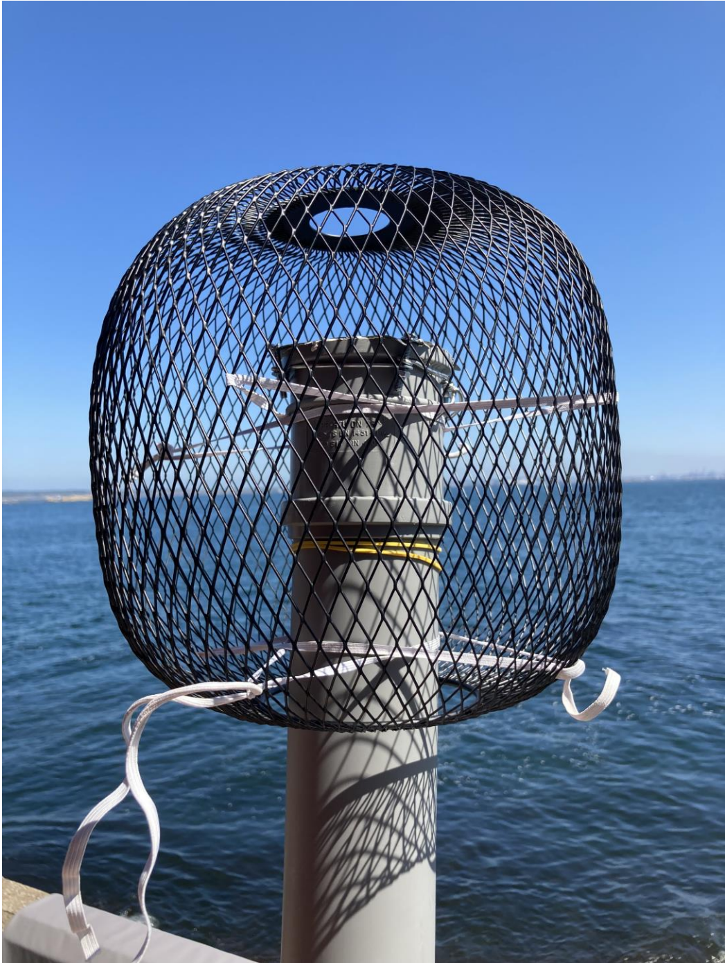
Figure 19. Wind shield frame for the low-frequency sensor. The frame was suspended with elastic bands to avoid structure borne sound.
