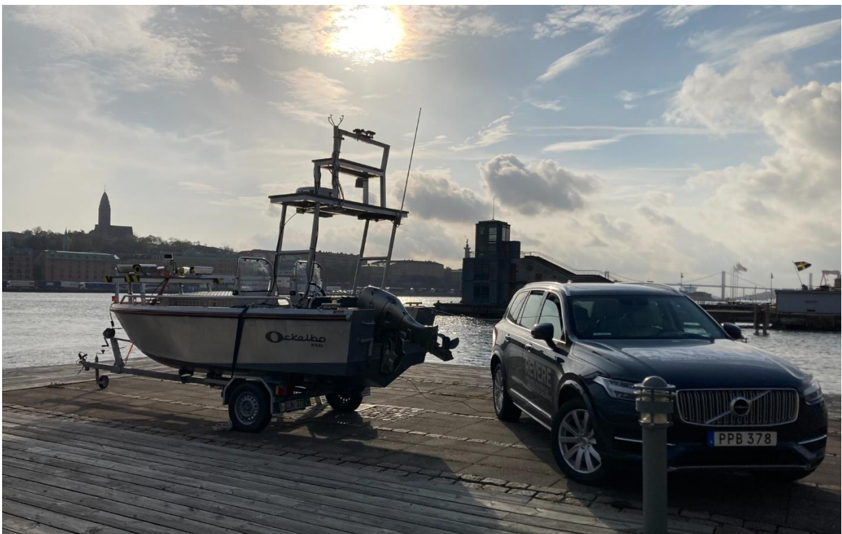
Image 13: Seahorse on a trailer, can also be utilised as a fixed shore sensor platform for a location that provides sufficient manoeuvring space for parking the trailer.
