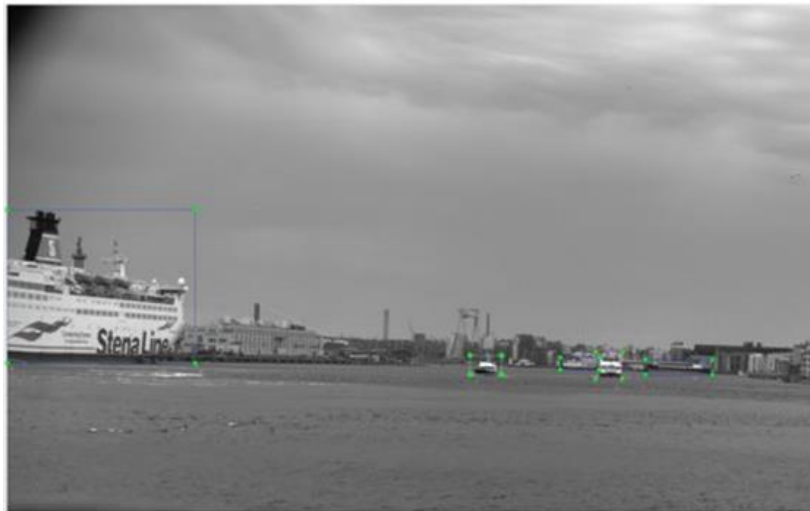
Image 17: An image object recognition algorithm being used to detect ships in the vicinity of Seahorse on one of the FLIR 4k cameras.
