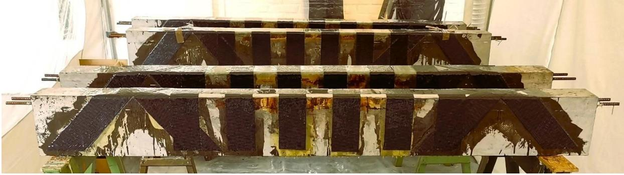
Figure 12: Combination of different FRP components from [8], with permission.
