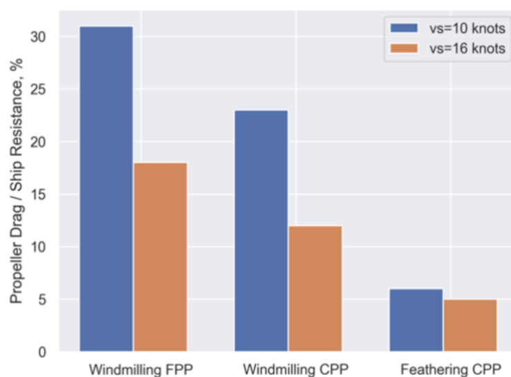
Figure 6. Propeller drag over ship resistance in windmilling and feathering positions.
