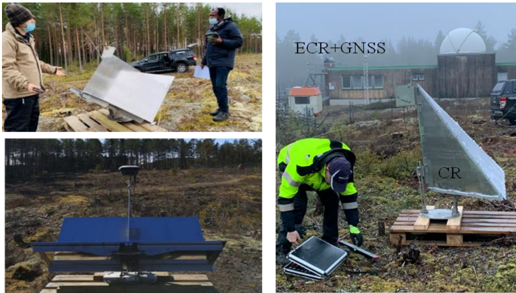
Figure 7, Experiments with corner reflectors in Mårtsbo test field. Learning how to orient triangular and double-back flipped squared types for Sentinel-1 ascending and descending tracks.
