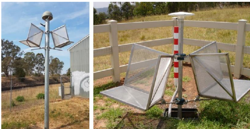
Figure 9, GNSS stations in the Sydney area with CRs attached to the antenna pole used by Fuhrmann et al. (2021).
