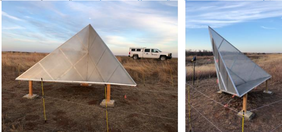
Figure 1, Two of the trihedral triangular corner reflectors installed in Texas for NISAR calibration (Information about Oklahoma and Texas NISAR Calibration Array can be found in the following link: https://uavsar.jpl.nasa.gov/cgi-bin/calibration-nisar.pl ).
