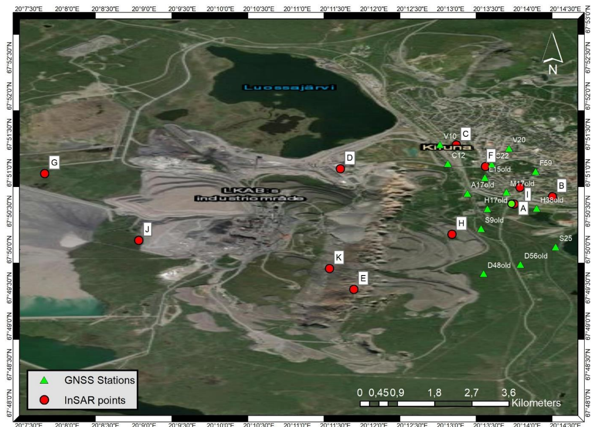
Figure 7. Location of the GNSS stations and InSAR points used for the cross-comparison over the Kiruna.
