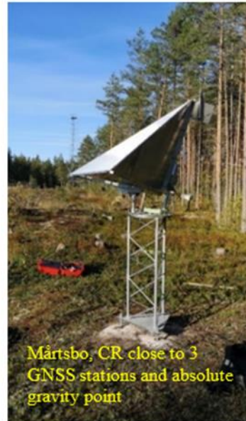
Figure 22, Different types of CRs installed at different locations (see Table 3 and Figure 8). Note the different shapes of the CRs and snow cover. The ones at Mårtsbo and Onsala are trihedral triangular types with inner leg of 1 metre and snow cover. The ones at Visby, are trihedral squared shape (trimmed version) with 1 m inner leg size, and snow cover. The ones at Östersund, Umeå and Skellefteå is double-backflipped squared shape with 72 cm inner leg and snow cover.
