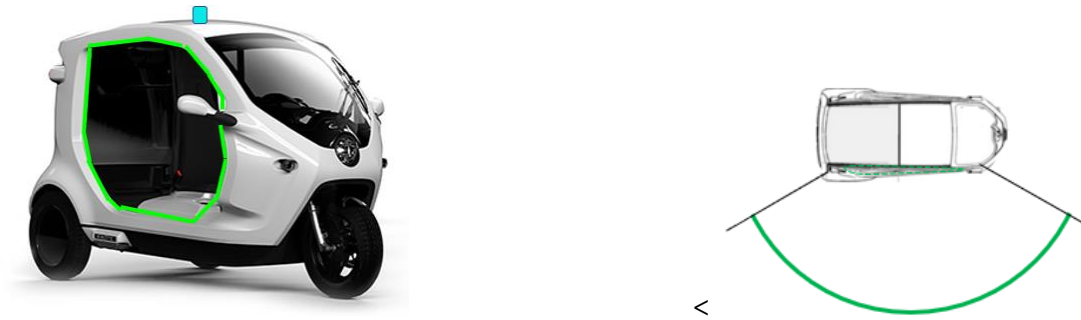
Figure 4, eHMI Load/Unload mode: LED-stripes mounted around the area where you load/unload goods. The Load/Unload mode was activated when the ADV had stopped for loading/unloading goods indicating that goods personnel could approach the ADV to load/unload goods.
