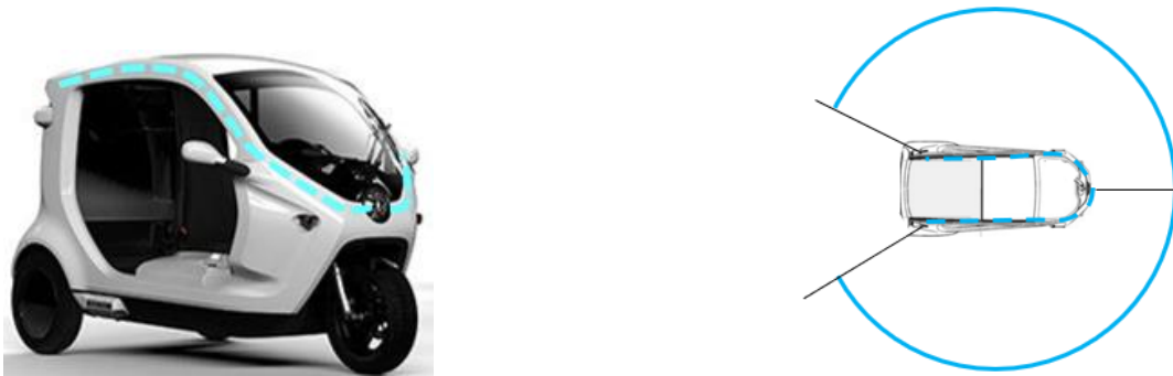
Figure 3, eHMI Deceleration/Acceleration: LED-strips mounted on the sides of the roof, along the A-pillars to the front lamp (same as the deceleration). During deceleration to standstill the lights were wandering forward from the roof's sides towards the front lamp. During acceleration from standstill the lights were wandering backward from the front lamp, along the A-pillars and over the sides of the roof. Colour: cyan.
