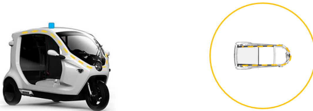
Figure 5, eHMI Unplanned stop: LED-stripes mounted on the sides of the roof, along the A-pillars to the front lamp. In the event of an unplanned stop the ADV (system) cannot solve but needs assistance the lights are flashing in yellow, together with the hazard lights on the vehicle. The eHMI for Unplanned stop was active until the situation was resolved.
