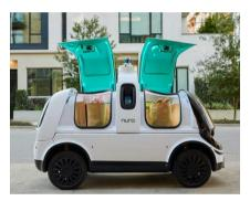
Specifications<sup>33</sup> Size: Length 274cm, width 110cm, height 186cm Loading capacity: 190kg Speed: 40km/h Weight: 1150 Kg
