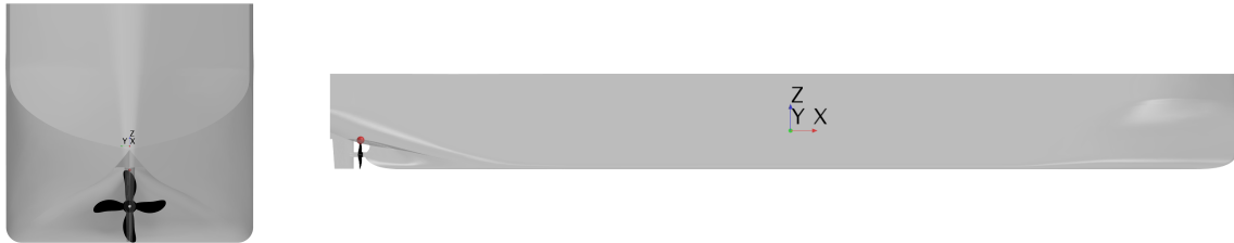
Figure 24: LDP vessel geometry, point probe and ship-fixed coordinate system at COG.
