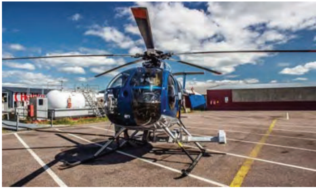
Figure 3. Picture of helicopter with measuring equipment used for 3D photography and laser scanning of the Iron ore line.
