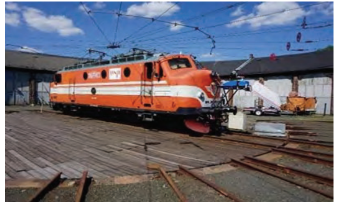
Figure 2. Picture of locomotive with measuring equipment used for 360 photography and laser scanning of the Southern iron ore line.
