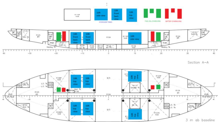
Figure 6 Suggested installation set-up before Hazard Identification workshop – showcasing case 3. The design consists of two FC units (green), two battery units (red) and six storage units (blue)
