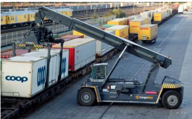
Figure 14: The reach stacker, a conventional technology commonly used for transshipment of unit loads at large intermodal terminals [Source: Coop]
