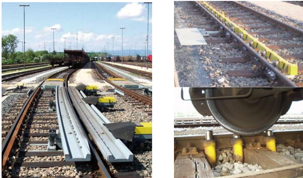
Figure 4: Automatic clasp (beam) retarder (left); Piston retarders in working position (right) [Source: wikipedia.org]
