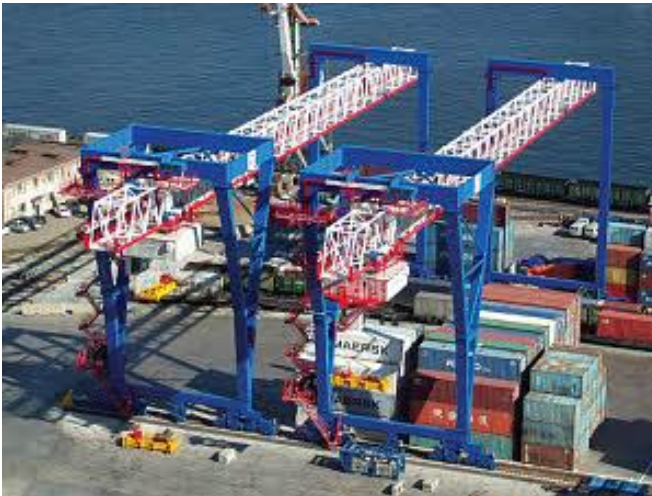
Figure 16: Rail mounted gantry crane a conventional technology used for transshipment and stacking of unit loads units at ports and large intermodal terminals [Source: Liebherr]
