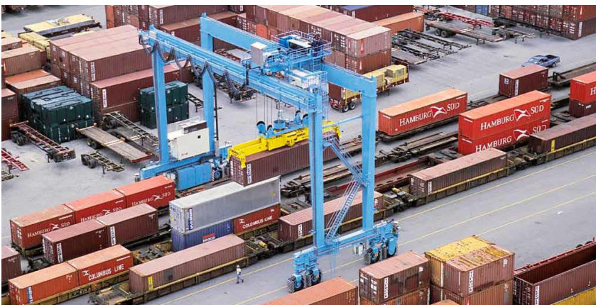
Figure 17: Rubber tired gantry crane used for transshipment and stacking of containers [Source: Liebherr]
