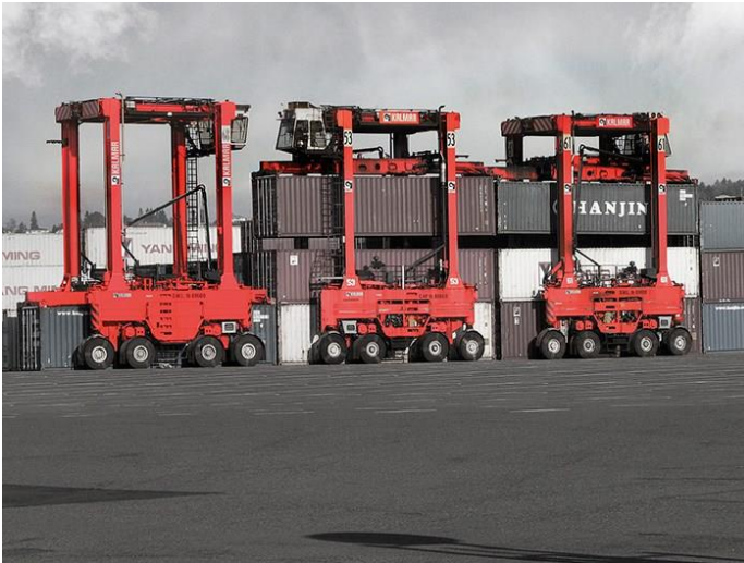
Figure 15: Straddle carriers used for stacking containers [Source: Kalmar industries]
