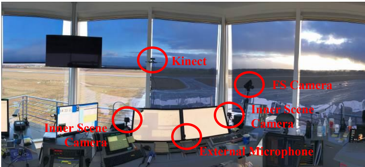
Figure 2: Overview of the CWP measurements at the example of Tower Tartu EENU in Estonia
