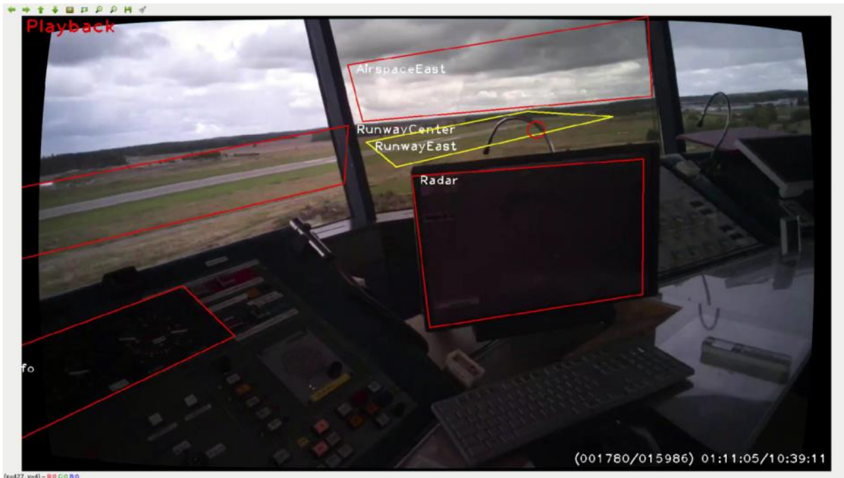
Figure 7: AoI Analysis example from Linköping ESSL (Project ETRA) with an automated detection of visual reference areas using AKAZE point features.
