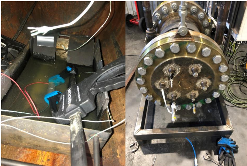
Figure 25. Pressure vessel seen from the inside (left) and outside (right).
