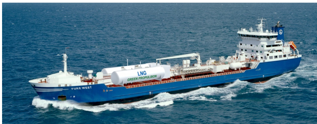
Figure 8. A photo of M/T Fure West with the LNG tanks digitally rendered (source: Kalantari et al., 2016).
