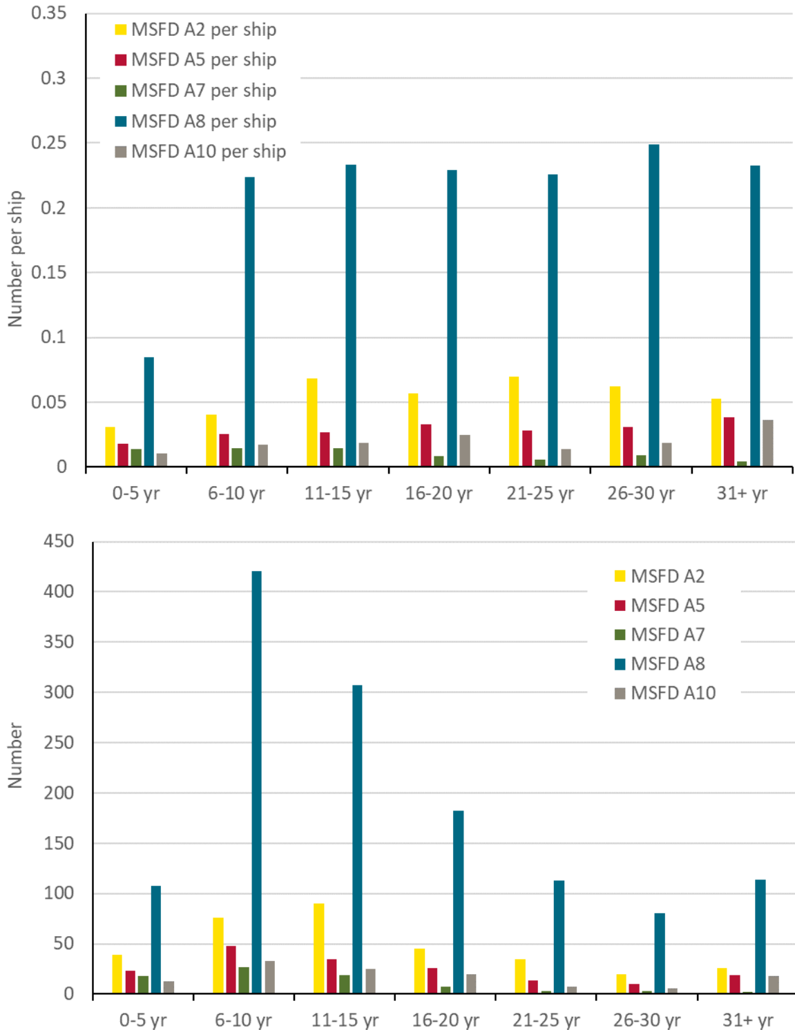
Figure 11. Number of deficiencies which can be related to five of the eleven descriptors of the Marine Strategy Framework Directive. Above: Number of MSFD A-related deficiencies per ship (i.e. total number of MSFD A-related deficiencies divided by total number of inspected ships in each ship age class). Below: Total number of MSFD A-related deficiencies.
