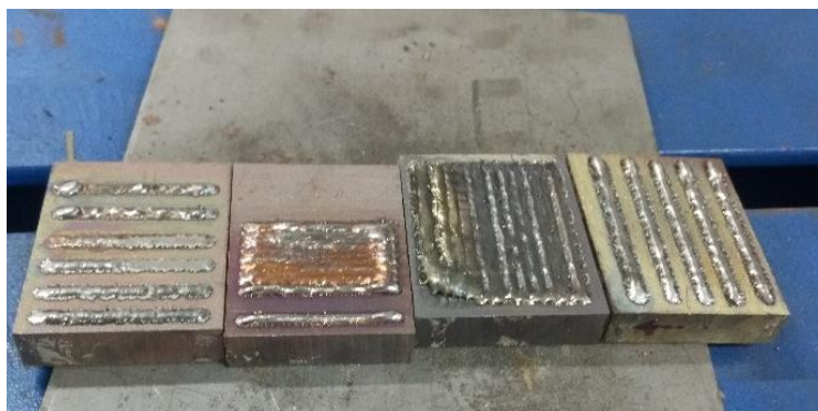
Fig.7: the test specimens from the pre-welding test.
