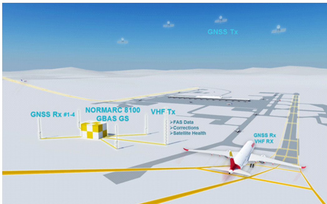
Figure 3 Illustration of the GBAS System.
