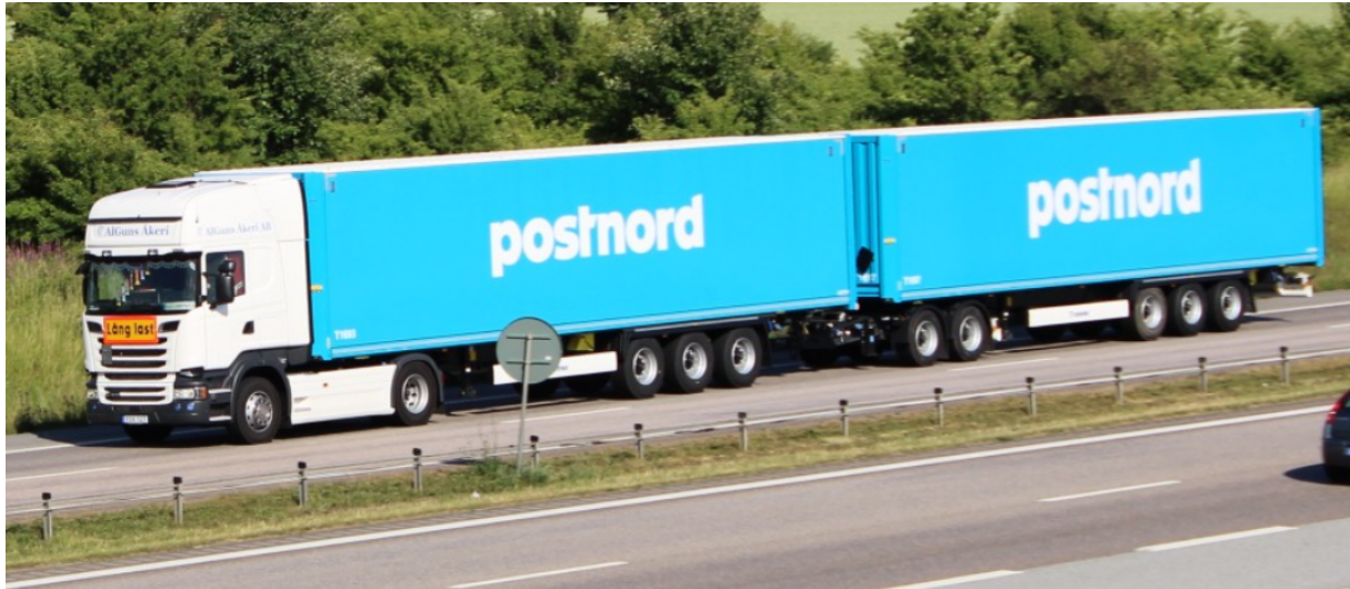
Figure 5.6 The duo trailer operating for PostNord. Note that there are only two axles on the tractor
