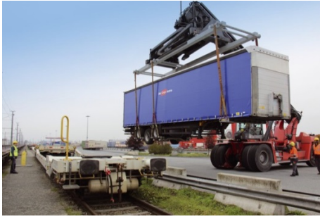
Figure 5.8 Transshipment of semi-trailer through cranes (Reach Stacker) or the Mega Swing wagon.
