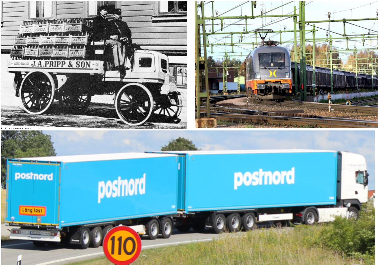
Figure 3.3 Examples of HCT-solutions: PostNord's 32m duo-trailer (bottom) and Hector Rail's TRAXX locomotive pulling a long and heavy train (top right). Compared to the first truck in Sweden (top left), the cargo capacity in a HCT truck is some 80 times higher at a low increase of fuel consumption per km.
