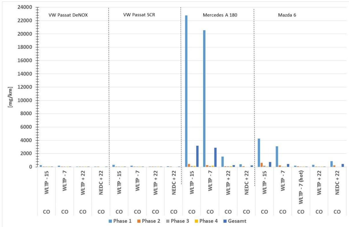
The emission of carbon monoxide is relatively low for all cars at tests at 22 C. The emission is highest for the gasoline car but the emission of HC only occur at the first part of the cycles and after catalyst converter reach the light-off temperature the emissions of CO is thereafter close to zero. For the three diesel powered cars the levels of CO emissions are low. For Mazda 6 the emissions seams to increase with decreased ambient temperatures.
