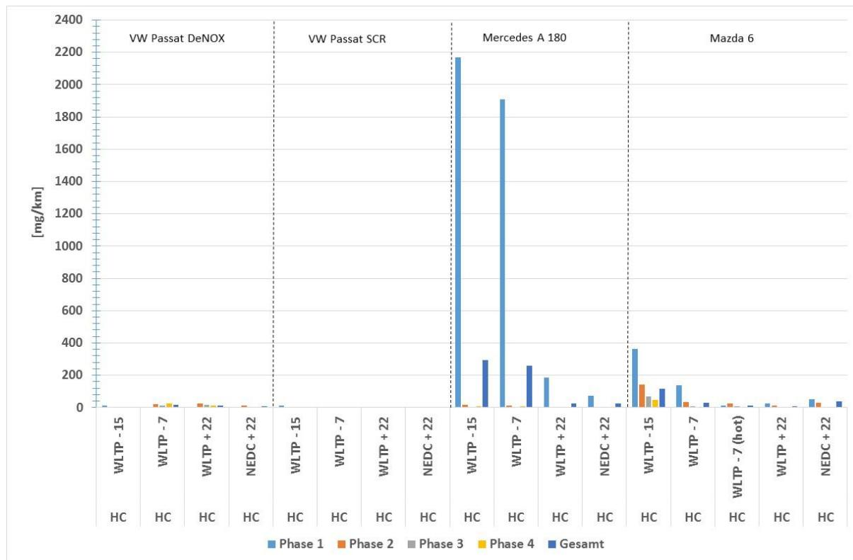
The emission of hydrocarbon is relatively low for all cars at tests at 22 C. The emission is highest for the gasoline car but the emission of HC only occur at the first part of the cycles and after catalyst converter reach the light-off temperature the emissions of HC is close to zero. For the three diesel powered cars the levels of HC emissions are low. For Mazda 6 the emissions seams to increase with decreased ambient temperatures.
