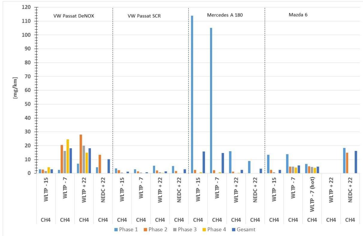
There is no limit value for methane in Euro 6. The emissions of methane is relative low during all tests except beginning of test cycle for the gasoline. But after catalyst converters reach the light-off temperature the emissions of methane is close to zero.
