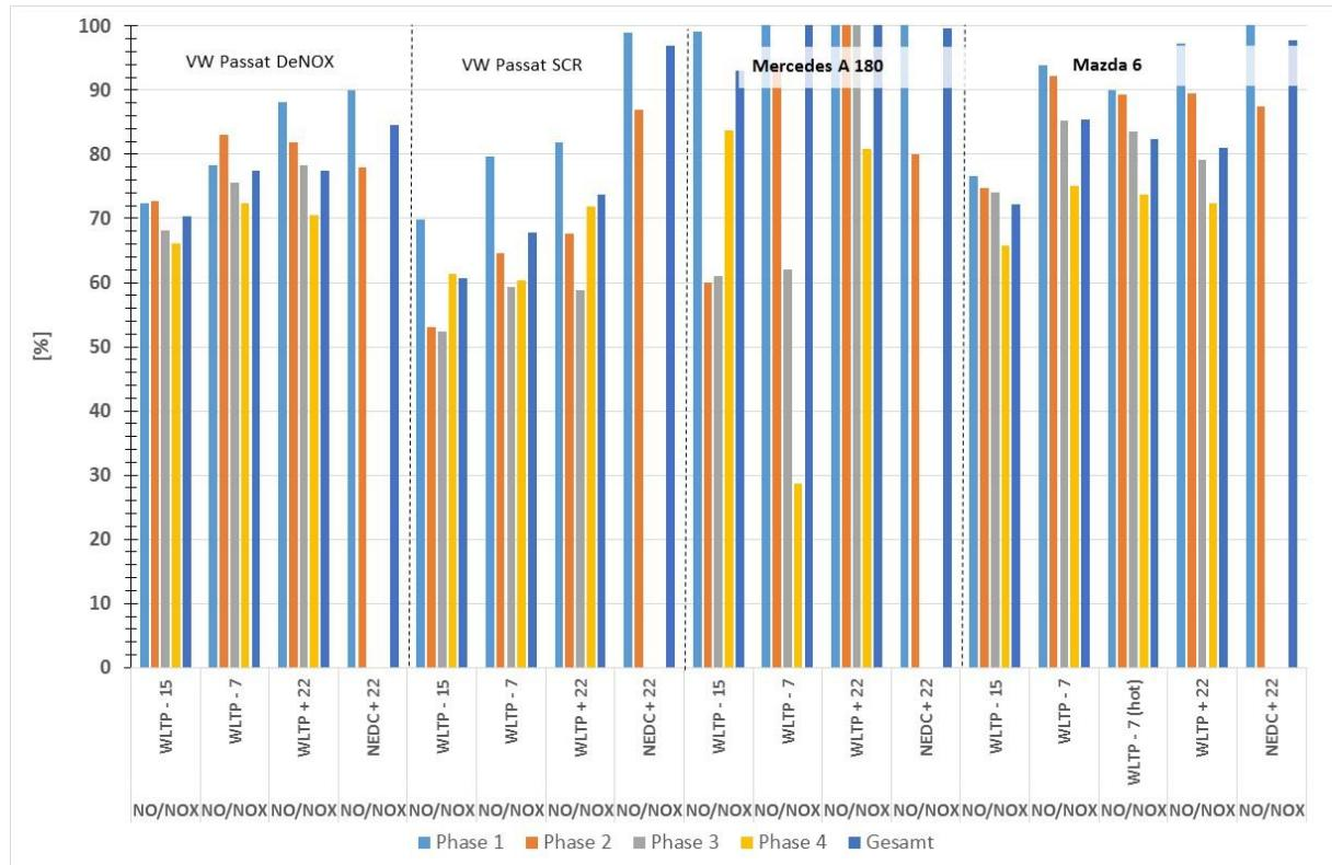
Interesting to note is that almost all NOx emitted consists of NO. For the gasoline car the NOx is more or less 100 % NO.
