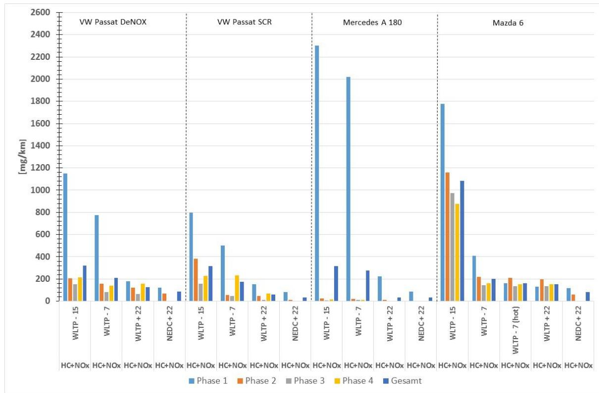
There is relatively high NO<sub>x</sub> + HC emissions for all tested diesel cars during test outside the NEDC (with certification conditions) test cycle. Especially at low ambient temperature the emissions are significantly higher than the Euro 6 limit.
