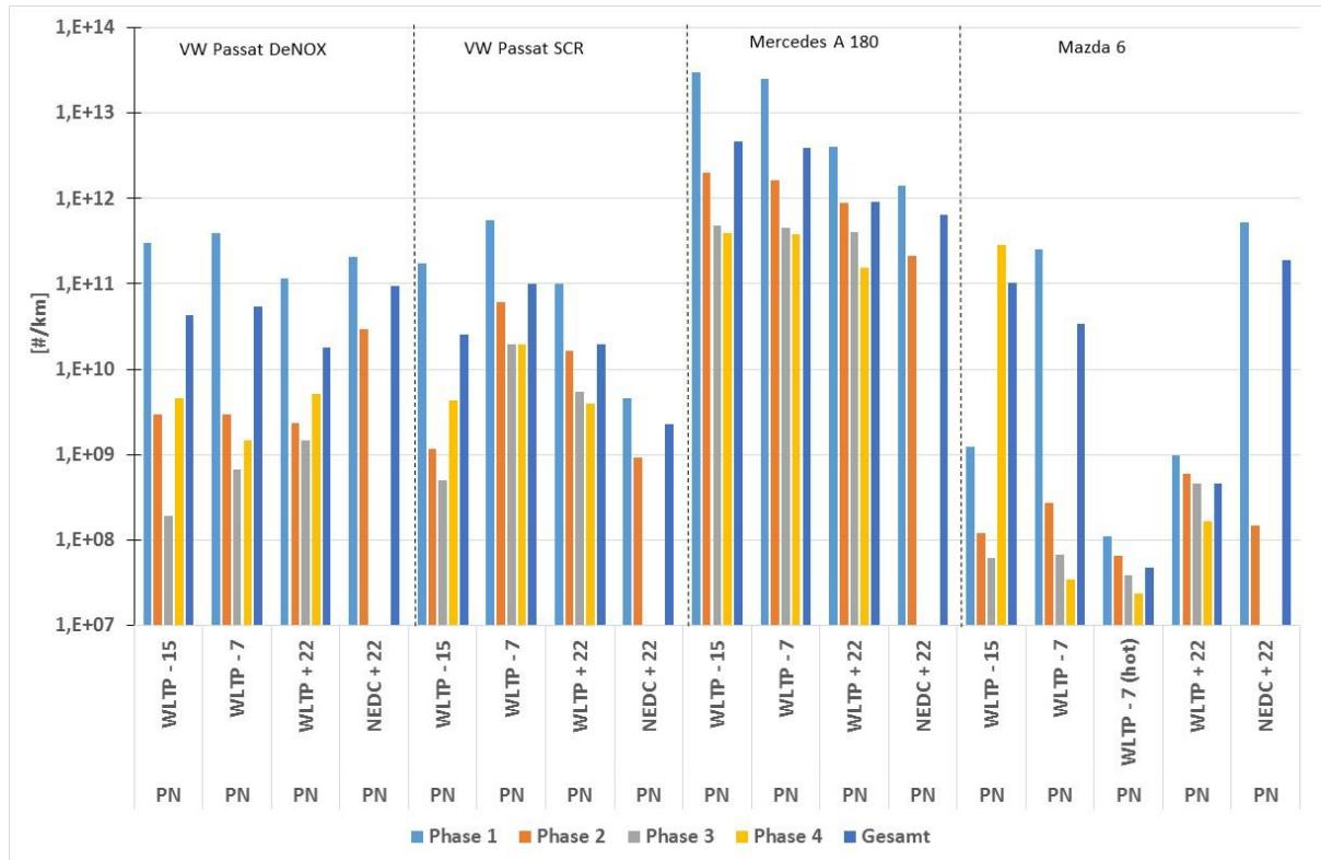
There are no significant differences in emissions of number of particles between the three tested diesel cars. The number of particles are higher with start at low ambient temperature but the behaviors are almost the same for all diesel cars tested.
