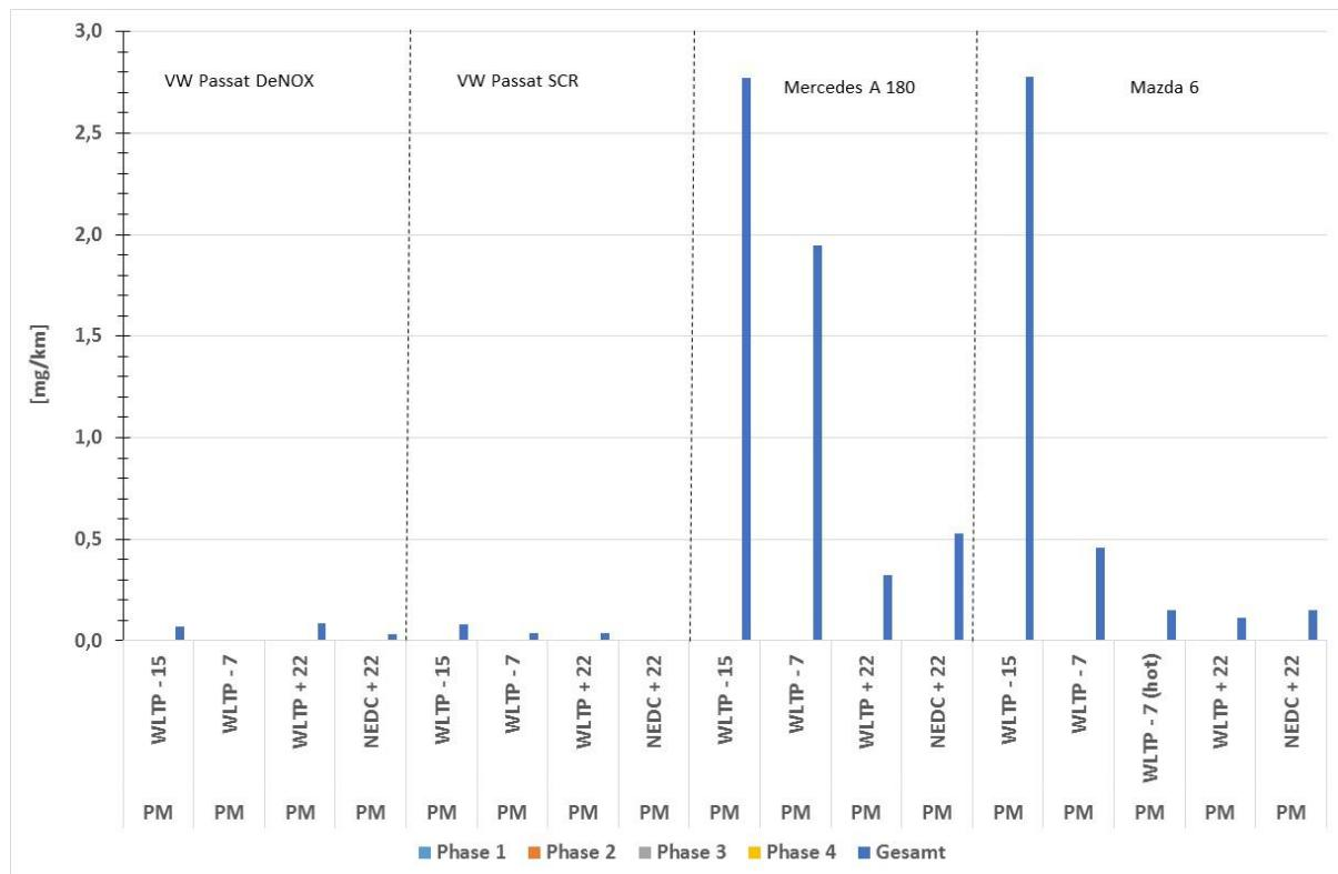
PM was measured by collecting particles on filter paper. These are very low weights (in absolute terms). This allows the measurement uncertainty is relatively large, so large that it is difficult to draw relevant conclusions from filter weight (e.g. for modern cars it is so low emission of particle mass that it is difficult to measure on filter). A general conclusion is that there are very low PM emissions. The Euro 6 limit is 5 mg/km and all car tested are well under the limit.
