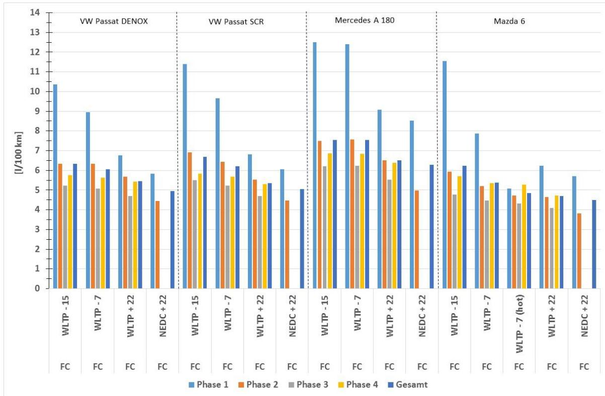
CO<sub>2</sub> and fuel consumption seems to be higher for WLTP compared with the NEDC test cycle and also increase with decreased ambient test cell temperatures.
