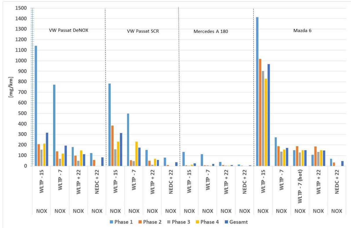
There is relatively high NOx emissions for all tested diesel cars during test outside the NEDC (with certification conditions) test cycle. Especially at low ambient temperature the emissions are significantly higher than the Euro 6 limit.
