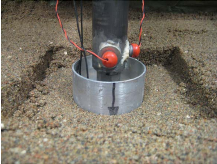
FIG. 2 – End of compaction with no observable heave.
