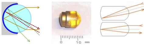
Figure 2. Left: Spherical retroreflector and reflection of three light rays. Center and right: Cat's eye glass body and principle of operation (back face is mirror-coated). Image credits: [3], [4]
