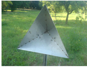
Figure 4. Example of a corner reflector used for radar testing. Image credit: [9].
