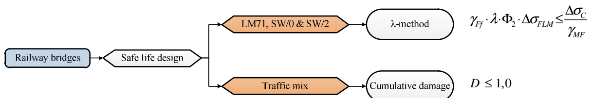
Figure 2.11 Fatigue design procedure of railway bridges
