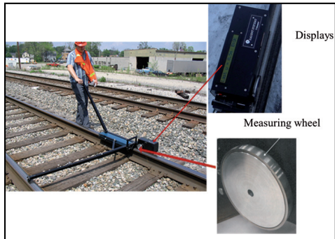
Figure 2. Schematically diagram of Tribometer
