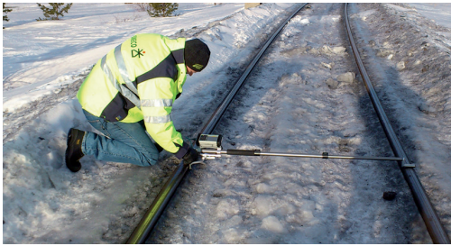
Figure 5. Field measurements with MiniProf on the southern part of the Iron Ore Line.
