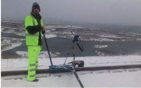
Figure 1. Demonstration of hand-pushed Tribometer
