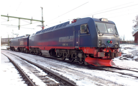
Figure 1. Two locomotives that pull 68 wagons with a gross weight of 8500 tonnage
