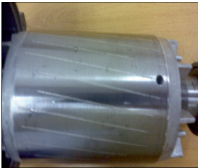
Figure 3b. One Broken Rotor Bar configuration
