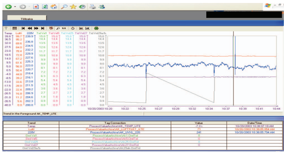
Figure 5.3.3 DISA interface for trending and correlating of different measurement data
