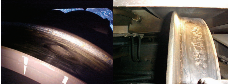
Picture 5.1.2. Left picture, wheel damage indicating peak value of 199kN, dynamic value of 96.3 (46 km/h). Right picture, wheel damage indicating peak value of 285.2kN, dynamic value of 185kN (79 km/h).
