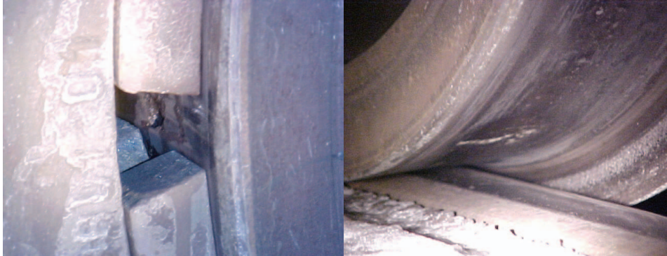
Picture 5.1.1. Left picture showing the damage identified between the brake pads. Right picture showing barely revealed wheel damage.
