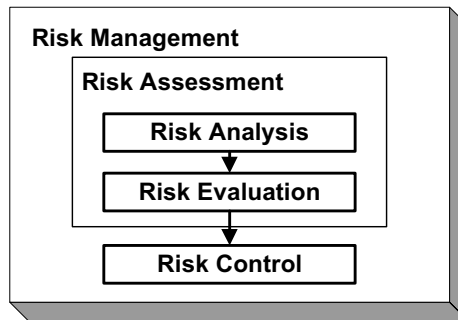
Figure 2.6. Risk Management consists of Risk Analysis, Risk Evaluation and Risk Control. Risk Analysis aims at identifying hazards, and at estimating the risk to individuals, populations, property, or environment. Risk Evaluation includes judgements of the tolerability of the risk on the basis of the Risk Analysis. Risk Control aims at managing and reducing the risk, and at implementing control activities in the organisation. (Source: IEC60300-3-9, 1995)
