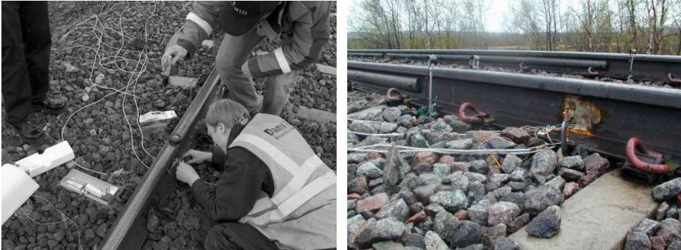
Figure 23. Installation of strain gauges for measuring vertical and lateral forces during the field test at Kiruna (Sweden).
