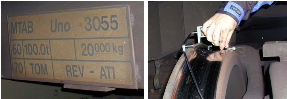
Figure 37. Picture of the measurement of wheel profiles on ore car Uno 3055 at the terminal in Luleå. [Courtesy: Damill AB.]
