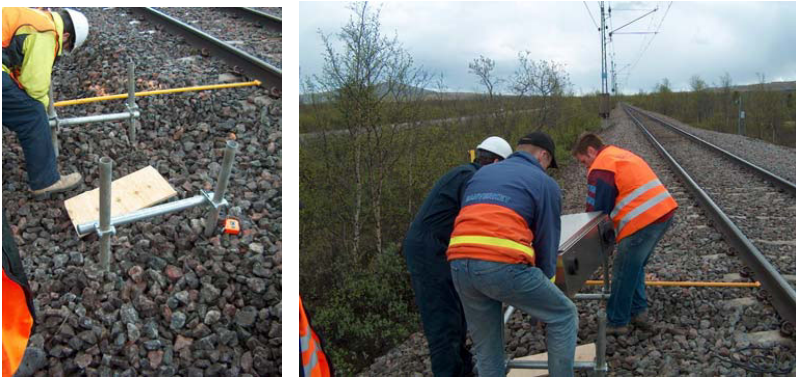
Figure 12. The four pipes in the ballast and the mounting of the monitoring equipment on to them during the field test at Kiruna (Sweden).
