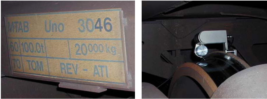
Figure 41. Picture of the measurement of wheel profiles on ore car Uno 3046 at the terminal in Luleå. [Courtesy: Damill AB.]
