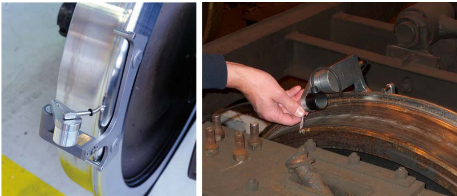
Figure 32. The MiniProf [Courtesy: Greenwood Engineering] is a handheld mechanical measurement tool for manual wheel profile measurements with very high accuracy. It was used as a reference tool in the test.
