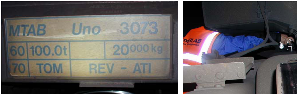
Figure 39. Picture of the measurement of wheel profiles on ore car Uno 3073 at the terminal in Luleå. [Courtesy: Damill AB.]
