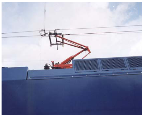
Figure 45. LKAB/MTAB iron ore locomotive IORE. (Sweden): Pantograph with automatic drop function to protect the interface when a failure occurs on the surface of the pantograph. [Courtesy: Rickard Granström]
