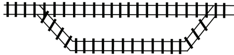
Figure 7 On a single track a station is used for meeting and overtaking trains.
