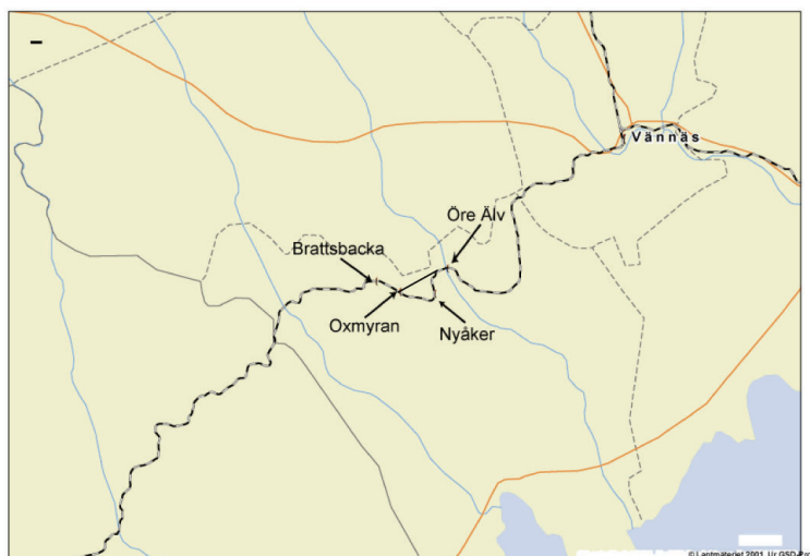
Figure 22 The main railway line from Vännäs to Oxmyran via Öre Älv and over Nyåker, and further south to Brattsbacka. The new track that was built in 1995 between Öre Älv and Oxmyran is marked as a straight black line between Öre Älv and Oxmyran.
