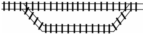
Figure 4. On a single track a station is used for meeting and overtaking trains.
