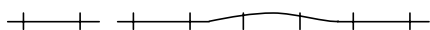
Figure A3. Old track laid with gaps in between rails, which are intended allow for temperature differences. If a gap is not wide enough, lateral buckling may occur. The gaps (exaggerated in the figure) give a characteristic sound when travelling.
