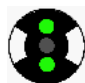
Figure A9. An announcement signal. Two flashing green lights mean “Expect 40” (km/h) (Banverket, 2002).
