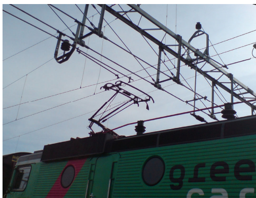
Figure A6. A pantograph of a Green Cargo locomotive receiving power from the contact wire at Älvsbyn station. The pantograph's two carbon slippers simultaneously touch the contact wire. Photo: Rikard Granström.
