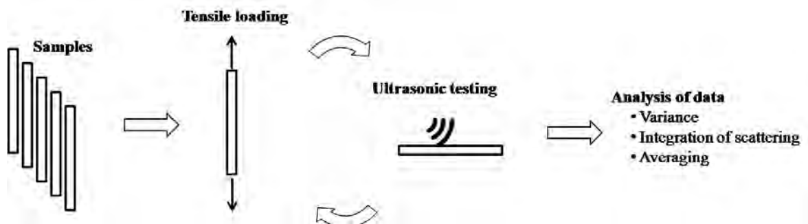
Figure 3.23: The experimental procedure.
