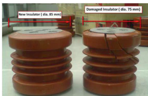
Figure 10: 85mm diameter size post insulators
