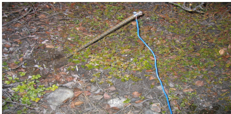
Figure 6. Iron rod attached to a copper wire used to measure the voltage difference between the iron rod and the S-rail.
