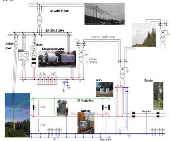
Fig. 1 Traction power supply system in Sweden
