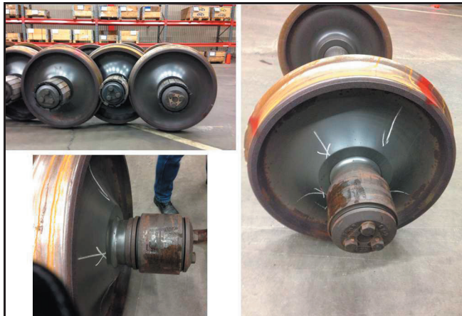
Figure 53. Inspection of the bearings before dismantling.
