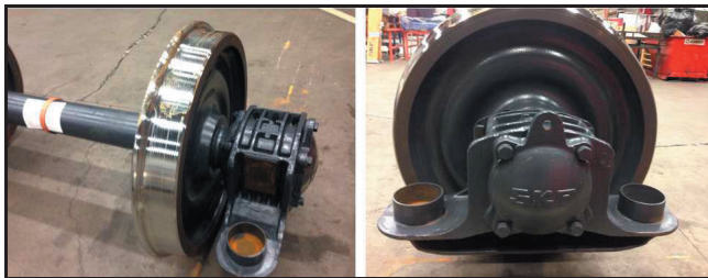
Figure 70. Assembled wheel with axle box.
