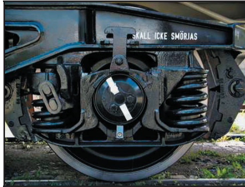
Figure 15. Y25 axle box assembly [46].
