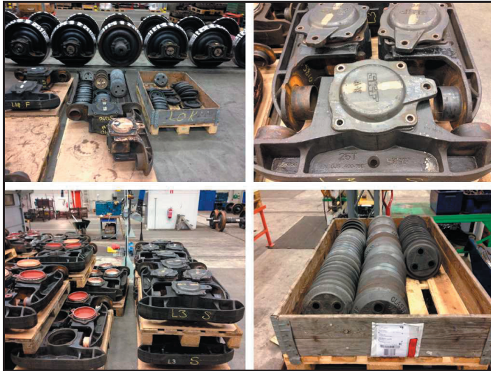
Figure 57. Axle box parts.
