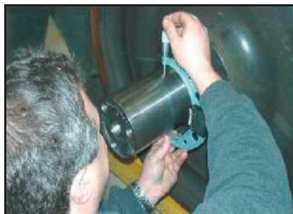
Figure 38. Bearing mounted lateral check using dial indicator [38].
