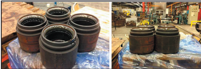
Figure 58. Outer ring of the bearings (presence of oxide on the surface).
