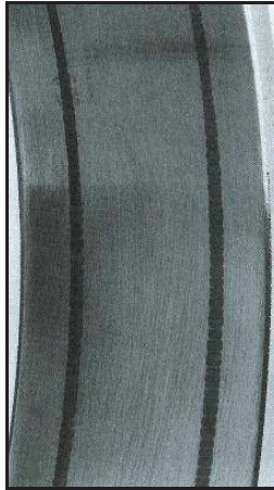
Figure 79. The outer ring of a self-aligning ball bearing damaged by electric current [41].
