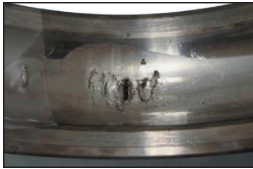
Figure 75. Excessive voltage. Ball bearing raceway with large spalls [47].
