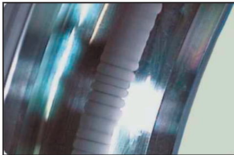
Figure 77. Fluting or washboarding in a raceway caused by the passage of damaging electrical current. Outer ring raceway of a deep groove ball bearing [47].
