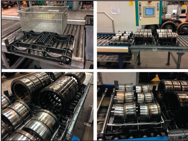
Figure 60. Rings and rolling elements on metallic frame.
