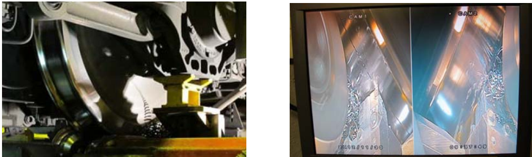
Fig.1.3 Locomotive wheel-sets undergoing on-site re-profiling
