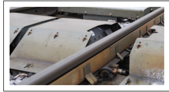
Figure 7. Picture of the rail and profile measurement system.
