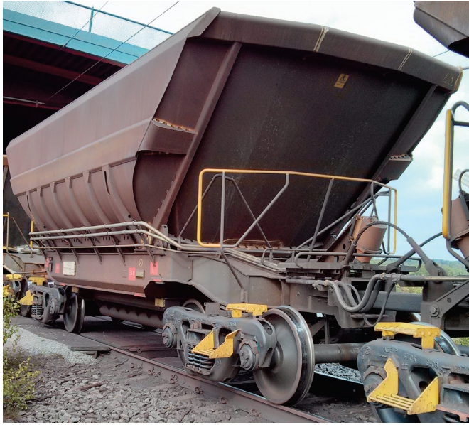
Figure 6.3: The Fanoo iron ore wagon
