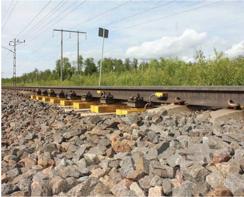
Figure 2: Wheel defect detector installed along the Iron Ore Line in the northernmost part of Sweden.
