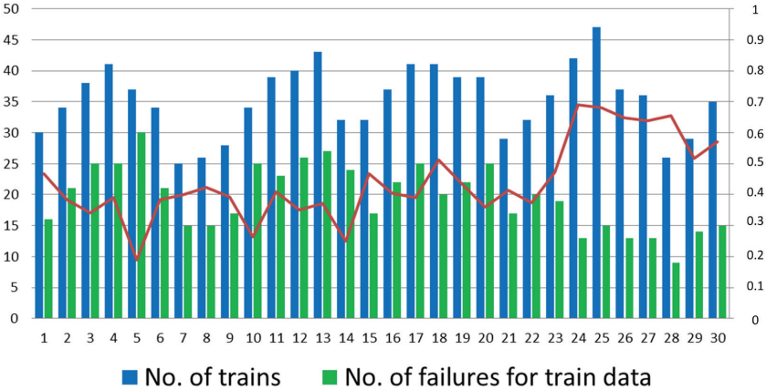
Figure 12: Measurement data from the WPMS for the month of April for the first year (2012); a process rate under 70% for each train means measurement failure.
