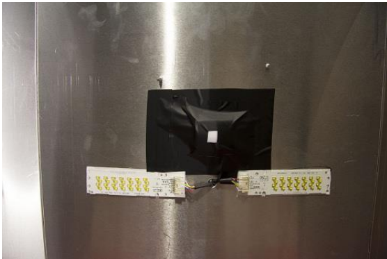
Fig.18 and 19: Both fixtures are equipped with 2x Philips Fortimo LED high brightness modules capable of reaching levels of 12,000\text{cd/m}^2 ( L_{\text{seq}} and L_{\text{th}} ) and one small LED source to reach low light levels as in the tunnel interior ( L_{\text{in}} ). The module on the right hand side is the one to fit in the front chamber where the user looks in; therefore it is equipped with an anti-glare reflector.
