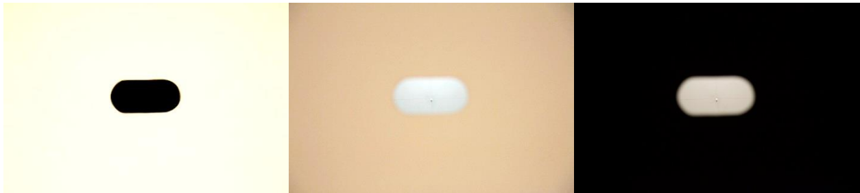
Fig.15 (1-3): Three lighting situations. To the left – front chamber fully lit (target is invisible). Middle showing equal (low) light levels in both chambers (target appears). Right hand showing dark front chamber and back chamber lit (target clearly visible).
