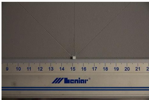
Fig.9 and 10: Show the target on the back surface (2x2x2mm) and the stereoscopic opening in the middle surface.
