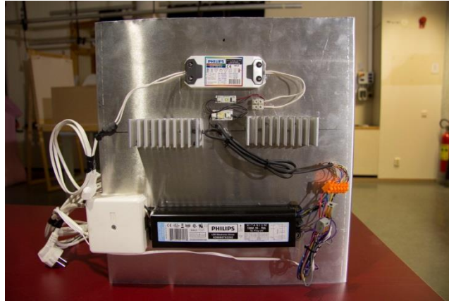
Fig.22: Top view of a complete module. Wiring and heat sinks exposed for easy control and better ventilation.
