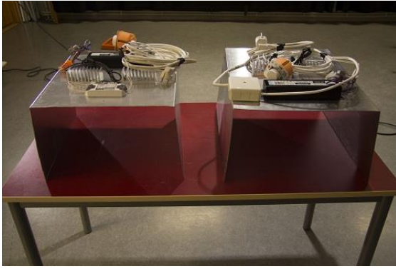
Fig.16 and 17: The custom made lighting structures. These fixtures mount on top of the model structure in the gap left open for them. The prevent external light spill and act as additional heat sinks.
