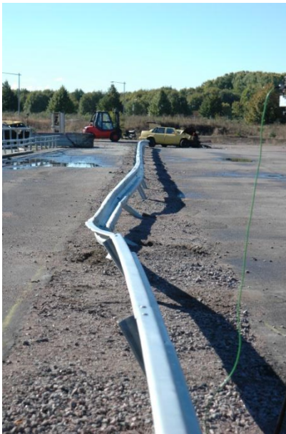
Barrier was too low and too angled, bolts did not shear off, resulting in a breach of barrier. Did see cracks and tear of the cross member.
