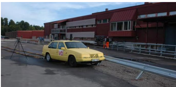
Figure 2. Test car at impact point using the 20° approach prior to collision test.
