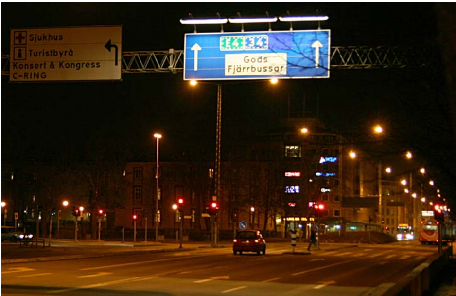
Figure 5 Vehicle headlamps, street lighting, traffic lights, commercial lighting, light from buildings, reflections and moon light all contribute to the total amount of light. The light level in the driving environment can thus vary a lot at night.
