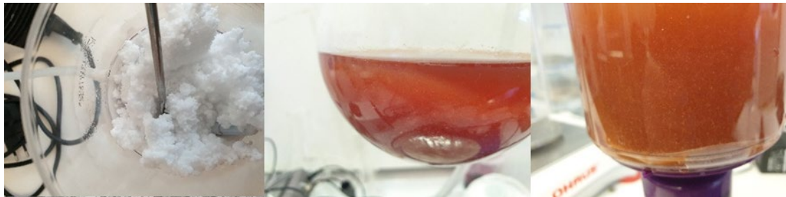
Figure 5. Experimental setup used for filtration of the synthesized capsules and filtered product
