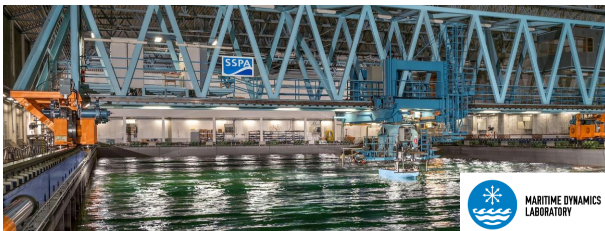
Figure 15: Seakeeping test in SSPA’s Maritime Dynamics Laboratory
