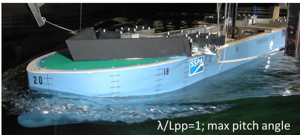
Figure 20. KVLCC2 model during seakeeping tests in “new” waves
