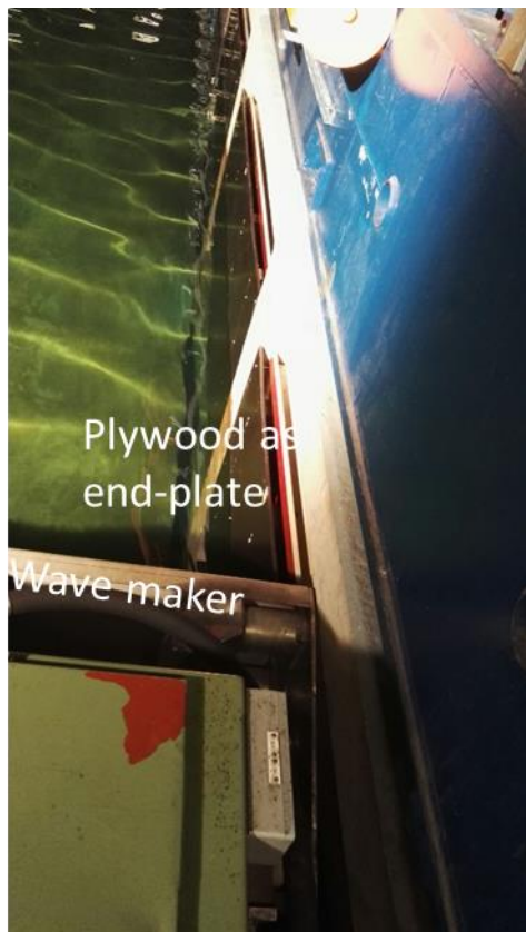
Figure 10: Added benefit; covers as an end plate sealing the end of the wave maker
