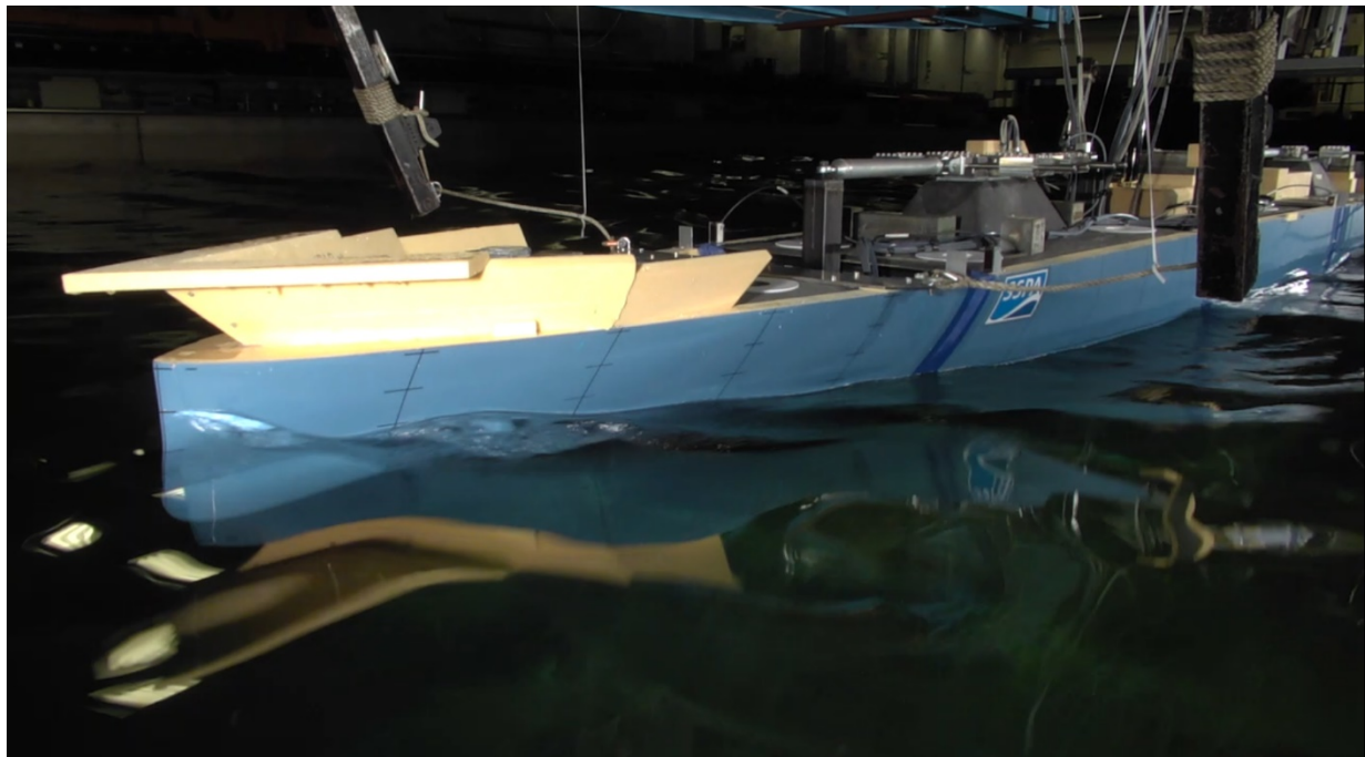
Figure 3.7: Seakeeping test run in SSPA MDL wave basin
