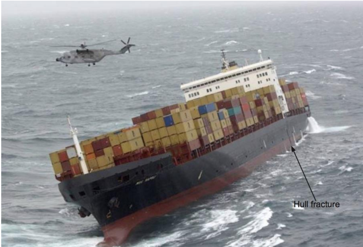
Figure 2. Photo from ref [12] showing some of the extent of the hull damage that led to scrapping of the container ship MSC Napoli after abandonment and beaching to prevent sinking.
