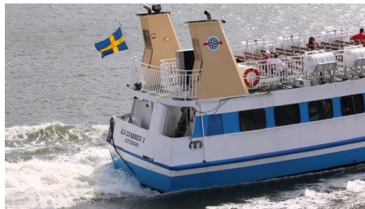
Figure 2. Älv-snabben 3 with a recirculating water region behind its transom (Photo: Arash Eslamdoost).
