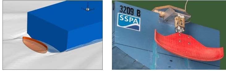
Figure 3. Placing of the Transom Pushing Device (TPD) in the computations (left) and the experiments (right)
