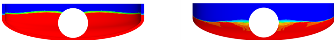
Figure 40. Wetted surface area of TPD used in waterjet. (left) concave side and (right) convex side of TPD.
